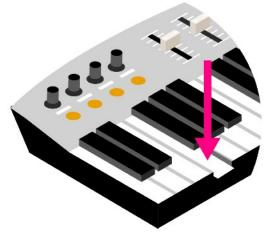
status: NOTE OFF 1° data byte: NOTE 2° data byte: VELOCITY NOTE OFF - When the key that was previously pressed is now released, a Note OFF message is generated that also consists of two numbers: pitch (0-127) and velocity (0-127) the key is released.
